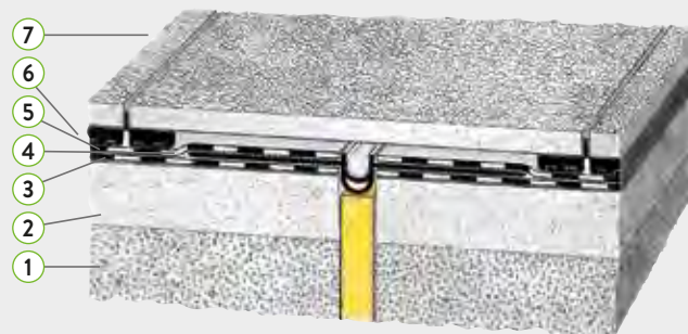
1 Deck 2 Lightweight concrete 3 Membrane 4 Elastic joint 5 Membrane 6 ITALPROFILI supports 7 Paving tiles
